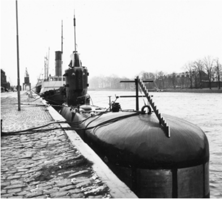
Anti-submarine nets were used in attempts to prevent submarines from penetrating areas that required protection, such as ports. But as is often the case in military contexts, such strategies breed counter-strategies. Submarines were equipped with net cutters to penetrate the nets. The Swedish submarine Makrillen with a net cutter in its bow, late 1960s.
