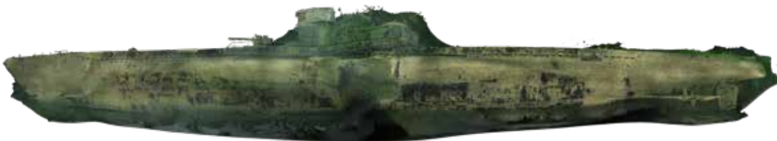
3D model of U-479 . The wreck lies at a 90-degree list at a depth of more than 90 metres in the Gulf of Finland. It bears traces of a powerful explosion to the hull at the command tower, probably caused by a mine.
