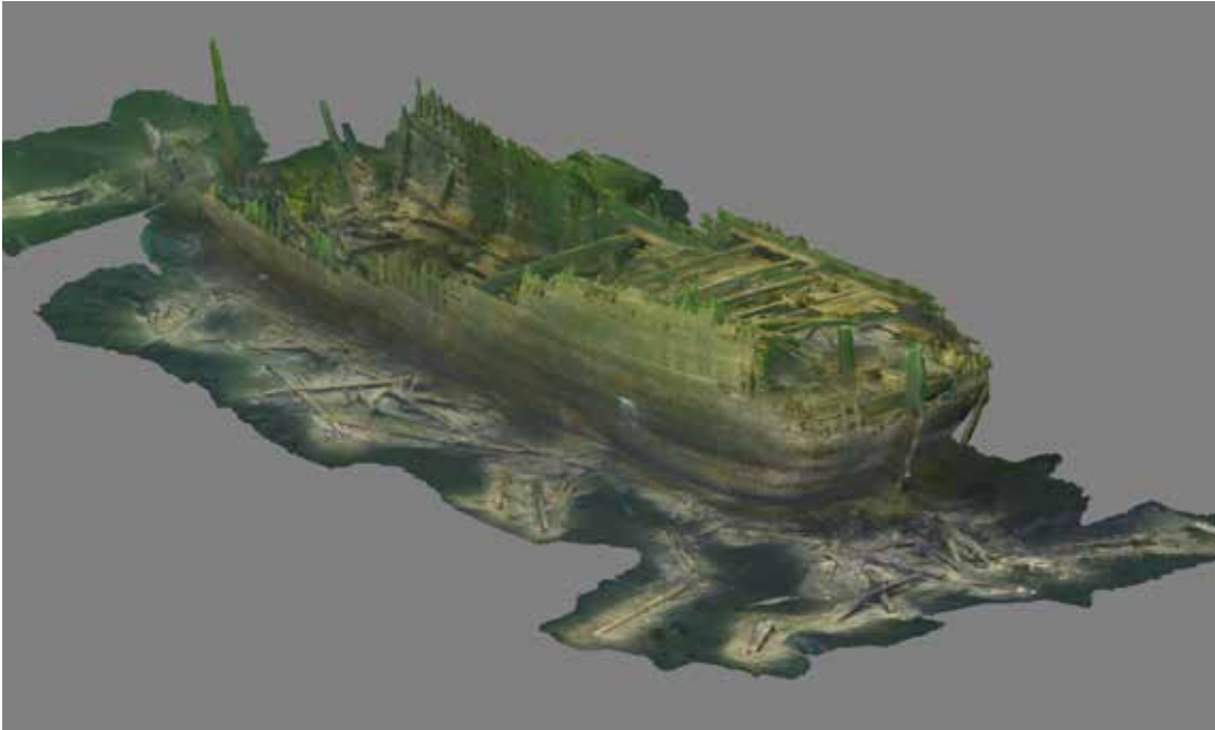
3D model of the wreck of the fluit ship Anna Maria , a merchant ship that caught fire in 1709 when it lay frozen in at Dalarö harbour. The wreck shows clear signs of fire damage.
